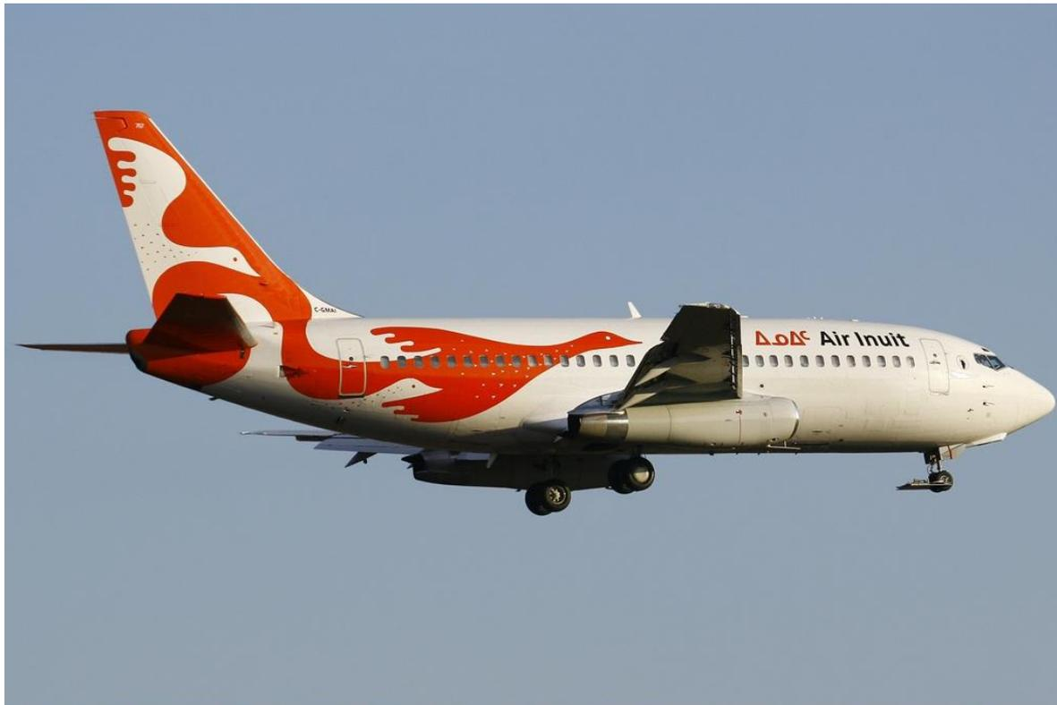
The 737-200s gravel kit, seen here with the nose gear deflector, is crucial for Air Inuit's Arctic operations.
